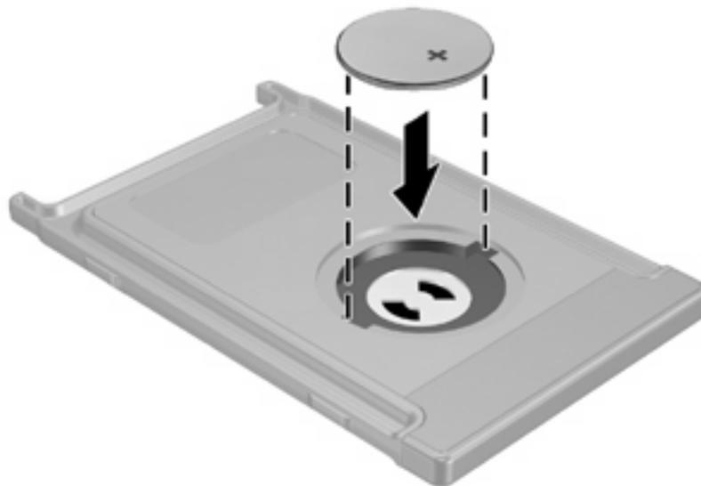
3. Insert the tabs on the battery compartment cover into the slots in the battery compartment and turn the cover clockwise to close.
