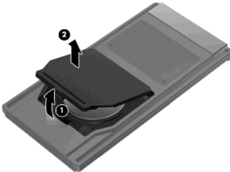
2. With the positive side of the battery facing up, insert the battery into the compartment (1).
