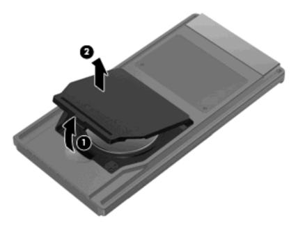
2. With the positive side of the battery facing up, insert the battery into the compartment (1).
