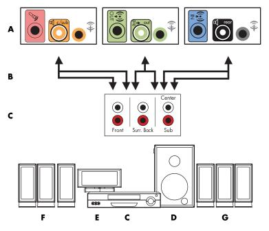
Computer to 7.1 multichannel audio system connection
