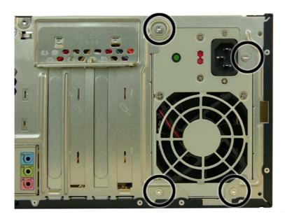
5. While pressing the tab in front of the power supply that holds it in place, pull the power supply up slightly to loosen it from the chassis.
