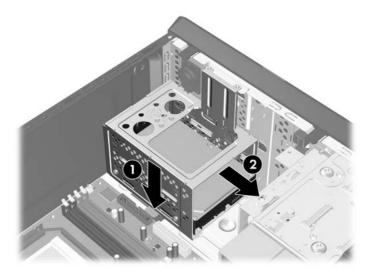
5. Lift the hard disk drive cage out of the chassis.
