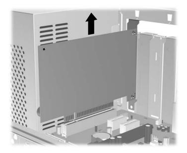
**c.** If you are removing a PCI Express x16 card, pull the retention arm on the back of the expansion socket away from the card and carefully rock the card back and forth until the connectors pull free from the socket. Be sure not to scrape the card against the other components.
