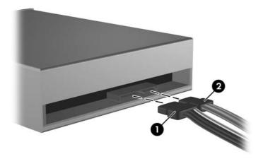
5. Remove the screws that secure the drive to the drive cage (1), then slide the drive out of the front of the chassis (2).
