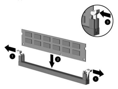
NOTE: A memory module can be installed in only one way. Match the notch on the module with the tab on the memory socket. A DIMM must occupy the black XMM1 socket.
