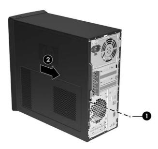
To install the access panel, reverse the removal procedure.
