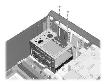
4. Push down the latch on the side of the hard disk drive cage (1), then slide the hard disk drive cage away from the bottom of the chassis (2) as shown below.
