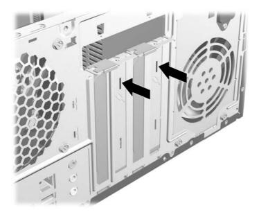
**b.** If you are removing a standard PCI card, hold the card at each end and carefully rock it back and forth until the connectors pull free from the socket. Be sure not to scrape the card against the other components.
