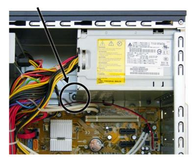
6. Lift the power supply out of the chassis.
