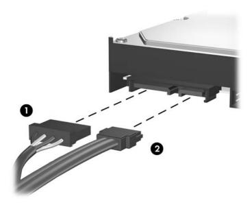
△ CAUTION: Never crease or bend a SATA data cable tighter than a 30 mm (1.18 in) radius. A sharp bend can break the internal wires.
