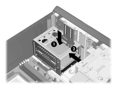
5. Attach the two screws that secure the hard disk drive cage to the chassis.
