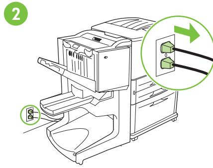
Disconnect the power cord for the printer from the AC power outlet. Disconnect the power cord for Tray 4 or the stand from the AC power outlet.
