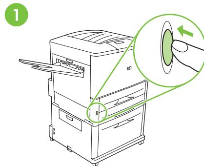
If you have already connected your printer to an AC power outlet, press the power button to turn the power off (button out).
