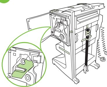
Position the device upright. Remove all foam and orange tape from the device. Remove the plastic bags from the cables.
