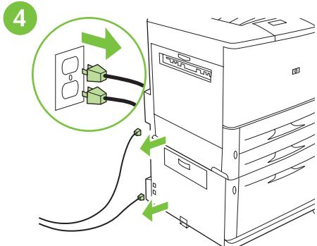
If connected, disconnect the power cords from the printer and Tray 4 and the AC power outlet.
