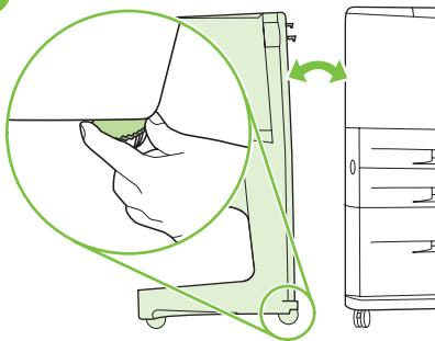
If there is a gap between the printer and the device, either at the top or at the bottom, adjust the blue levelers above the device wheels until there is no gap. Follow the label instructions above the wheels.
