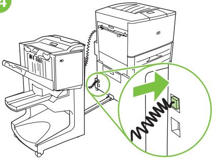
Connect the power cord on the device to the upper connection on Tray 4 or stand.
