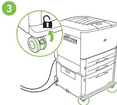
Unlock the printer front wheels.
