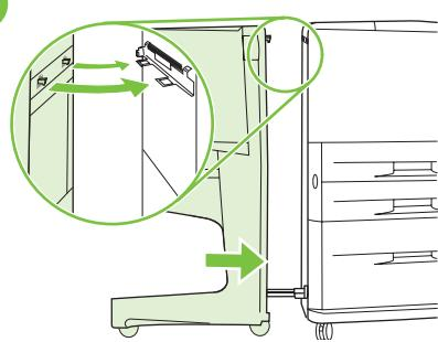
Push the device toward the printer. The two plastic hooks on the device should lock onto the latching bracket.
