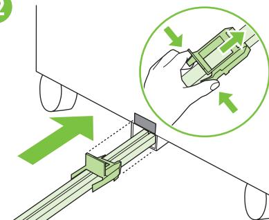
Slide the blue plastic bracket into the metal slot until it locks into place.
