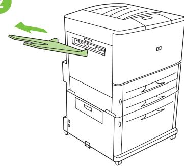
Remove the face-up bin (if installed) and store it. It is not used when the multifunction finisher is connected to the printer.
