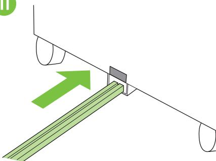
Put the end of the connecting rod into the U-shaped metal slot on Tray 4 or stand, and align the rod with the gray alignment label.
