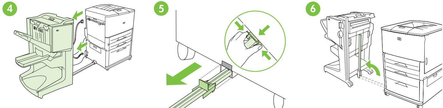
Disconnect the device's power cord from Tray 4 or the stand, and disconnect the communication cable from the printer.
