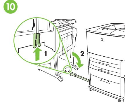
Slide the blue bracket up to unlock the rod. Lower the connecting rod to a horizontal position.
