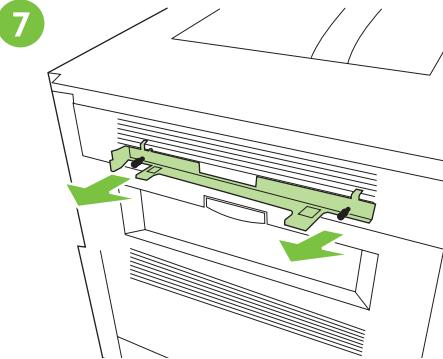
Unscrew the latching bracket from the printer.
