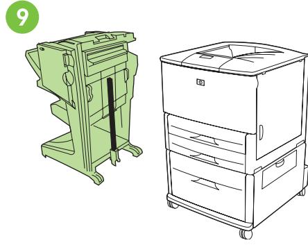
Position the device to the left side of the printer.
