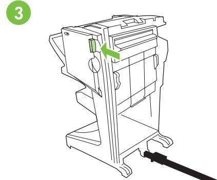
Press the release handle and move the device away from the printer.
