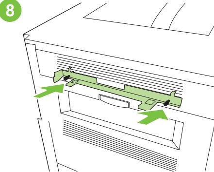
Position the latching bracket in front of the printer's cap holes and attach the bracket by reinserting the screws.
