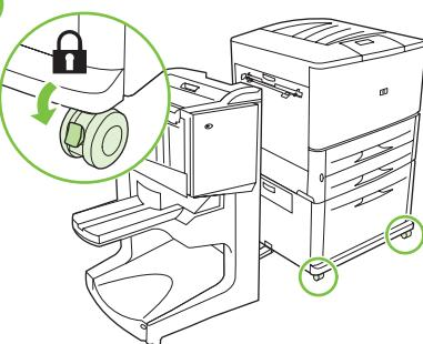
Position the printer in its permanent location, and lock its front wheels.
