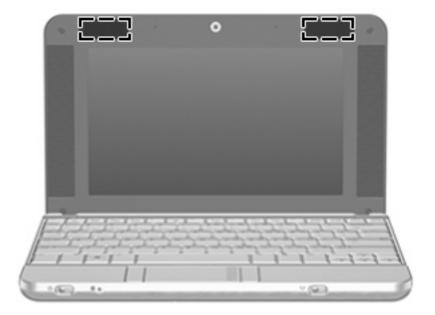
NOTE: For optimal transmission, keep the areas immediately around the antennae free from obstructions.
