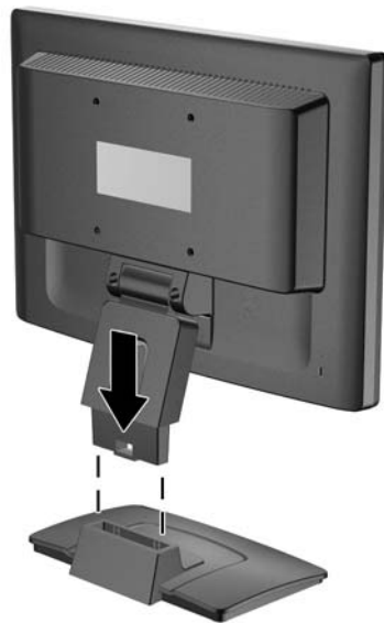
Figure 3-1 Attaching the Base to the Monitor
