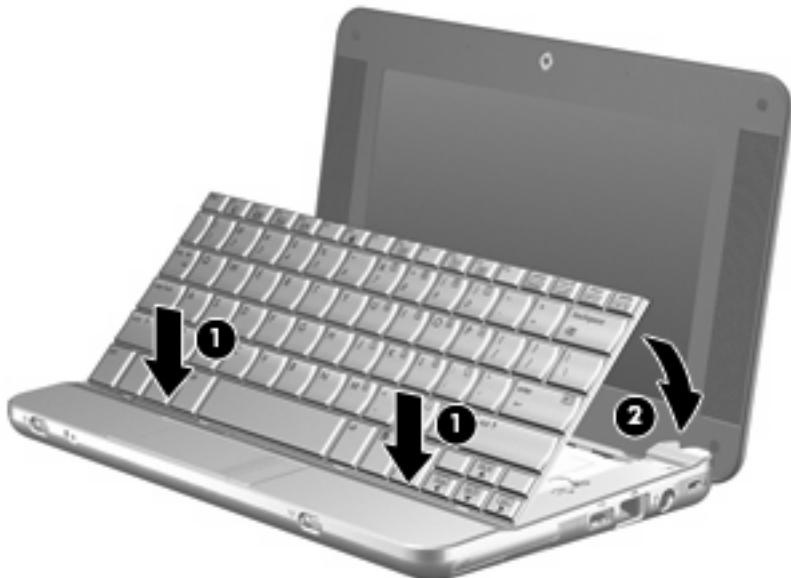
13. Close the computer display and turn the computer upside down on a flat surface.
