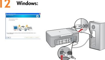
Windows: Once the USB prompt appears, connect the USB cable to the port on the back of the product, and then to any USB port on the computer.
