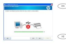
**Problem:** (Windows only) The **Device Setup Has Failed To Complete** screen displays. **Action:** Unplug the product and plug it in again. Make sure that the printer is turned on. Check all connections. Make sure the USB cable is plugged into the computer. Do not plug the USB cable into a keyboard or a non-powered USB hub. Refer to Step 12.
