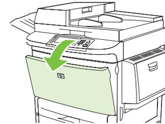
6 Check for paper in the duplex printing accessory area, and remove any paper by pulling it out of the MFP. Be careful not to tear the paper.
