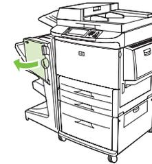
5 Turn the bottom green knob clockwise to advance the jammed paper through the folding rollers and into the booklet bin.
