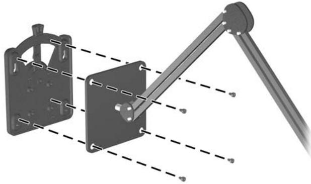
△ **CAUTION:** The Quick Release can also be installed directly to a wall to mount the monitor panel. It is designed to support a maximum of up to 24 lbs. (10.9 kg). If you are mounting to a wall, HP recommends that you consult with a qualified engineering, architectural, or construction professional to determine the appropriate type and quantity of mounting fasteners required for your application and to ensure that the mounting solution is properly installed to support applied loads.
