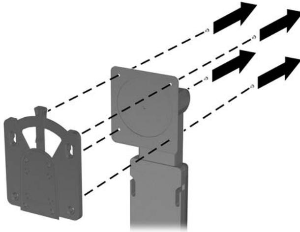
3. Mount the Quick Release to a swing arm or other mounting fixture using the four screws removed from the Quick Release in the previous step.
