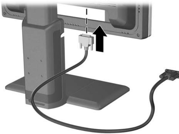
**Figure 3-4** Connecting the DVI-D Signal Cable
