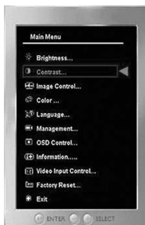
3. To navigate through the OSD Menu, press the **+** (Plus) button on the monitor's front panel to scroll up, or the **-** (Minus)/Auto button to scroll in reverse.
