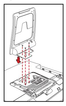
2 Replace the memory cover. Align the memory cover over the two legs of the computer stand and the screw hole and slide toward the stand and into place (A). Push down on both sides of the bottom edge of the memory cover to snap it into place (B). Push in the middle of the bottom edge to make sure the entire cover is pushed all the way down.
