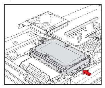
10 Disconnect the power and data cables by pressing the latches and then removing them from the drive.
