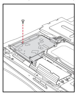
8 Remove the screw that secures the hard disk drive cage to the chassis.
