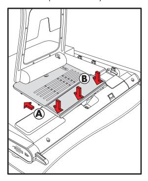
3 Replace the screw that secures the memory cover to the computer.
