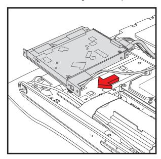
7 Replace the screw that secures the optical disc drive to the chassis.
