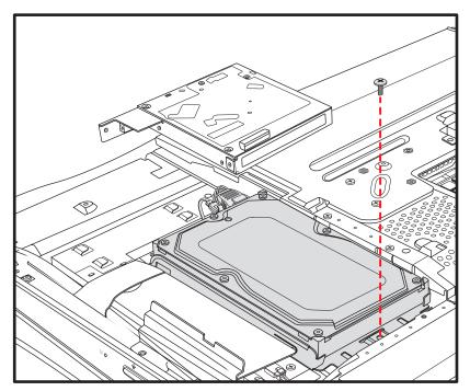
6 Align the hooks on the optical disc drive with the holes on the computer, and then slide the optical disc drive toward the outer edge of the computer.
