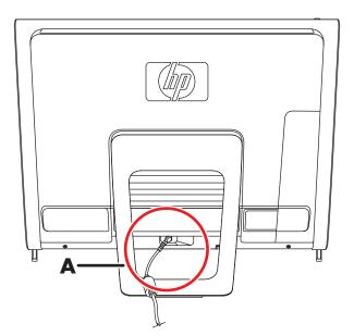
5 Remove the connector cover by inserting your finger under the gap on the bottom-left side of the cover (A), and then pulling gently.
