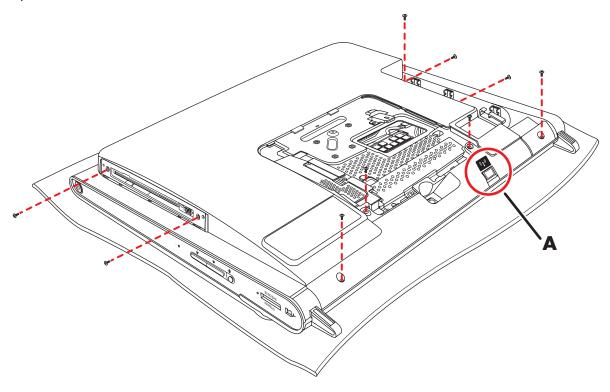
5 Lift the back cover up from the bottom inside edge of the memory cover area to release it, place both hands under the bottom edge of the cover and lift it up, and then rotate the back cover up as far as it will go.
