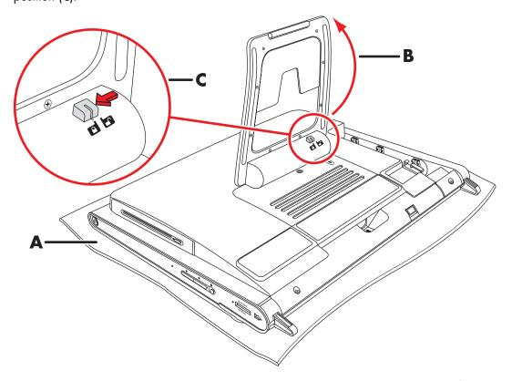
**9** Using the notch on the wireless keyboard and mouse receiver, pull the receiver out of and away from the back of the computer.
