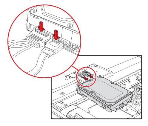
4 Lower the hard disk drive cage straight down, align the four hooks on the cage with the four holes on the back of the chassis, and then slide the cage toward the bottom of the computer until it rests against the bracket on the chassis.
