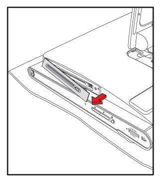
4 Make sure the wireless keyboard and mouse receiver (A) has been removed. See "Opening the HP TouchSmart PC" on page 3. Remove the nine screws that secure the back cover to the chassis. Four of the screws are located along the bottom edge of the back cover, two are located on the sides of the optical drive, and three are located in the connector area.
