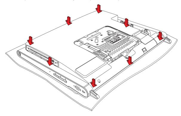
10 Replace the nine screws that secure the back cover to the computer. Four of the screws are located along the bottom edge of the back cover, two are located on the sides of the optical drive, and three are located in the connector area.
