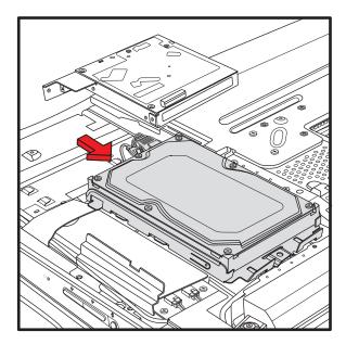
5 Replace the screw that secures the hard disk drive cage to the chassis.
