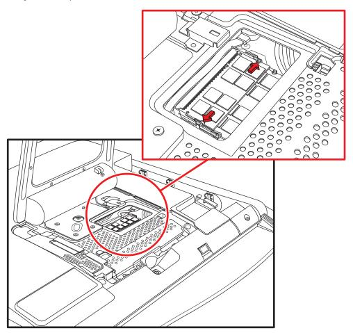
Lift the memory module from the memory socket. Note the location of the key slot on the connector edge.
