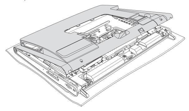
**9** Press the top, side, and then bottom edges to snap the cover into place.
