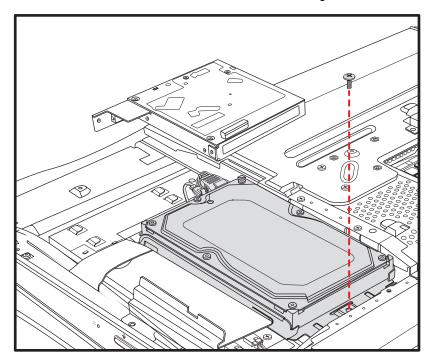
9 Slide the hard disk drive cage toward the top of the computer, and then pull it away from the computer.
