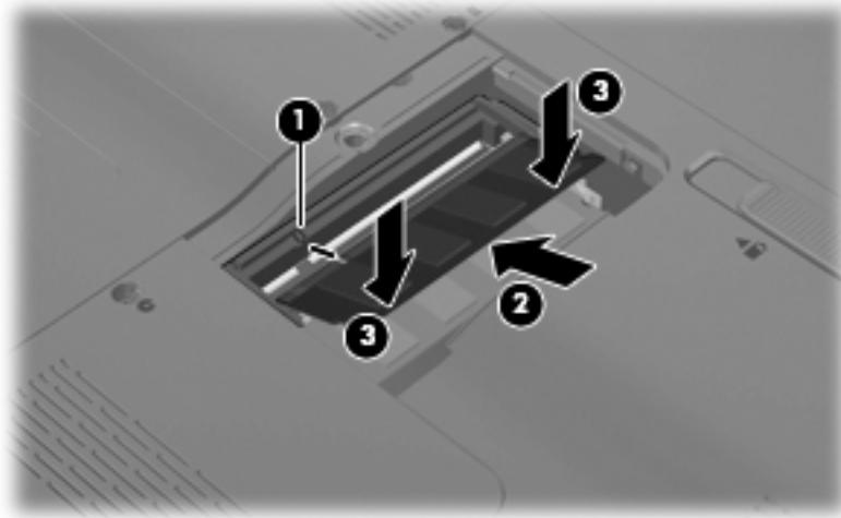
11. Align the tabs (1) on the memory module compartment cover with the notches on the computer.
