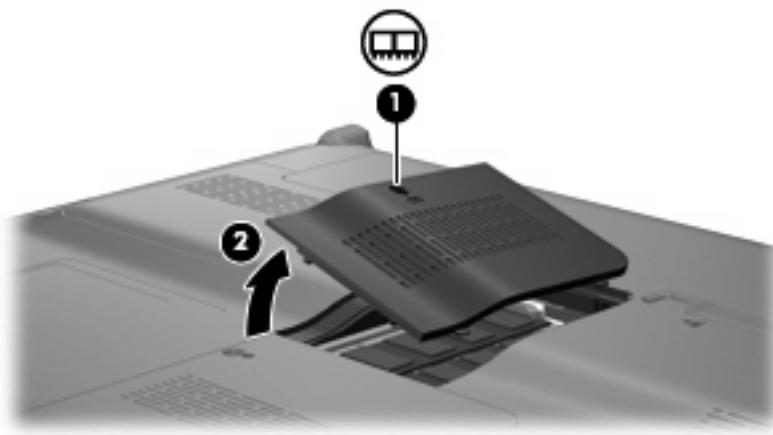
9. If you are replacing a memory module, remove the existing memory module:
