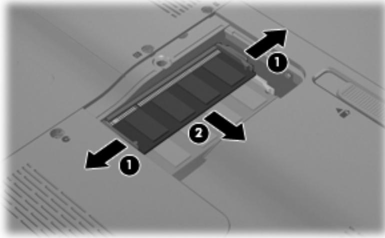
To protect a memory module after removal, place it in an electrostatic-safe container.
