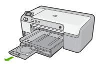
Securely snap the inkjet printable media onto the CD/DVD holder with the printable side up. The CD/DVD should be placed on the ring at the end of the holder with the arrows.
