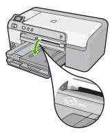
Make sure you loaded a printable disc onto the CD/DVD holder with the printable side up. Push the CD/DVD holder forward into the CD/DVD tray until the lines on the holder line up to the white lines on the tray. The end of the holder marked with arrows goes into the CD/DVD tray first.
