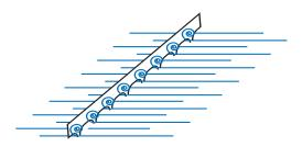
3. When a headstrike occurs, those sharp orifice projections scrape printed ink and media particles and drive the particles into the orifices themselves.
