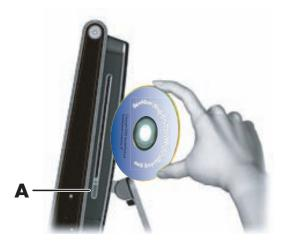
To eject a disc, make sure the power is on, and then press the eject button (**A**) on the side of the disc drive. You can also tap the **Windows Vista start button**, tap **Computer**, press and hold (or with the mouse, right-click) the optical drive, and then tap **Eject**.
