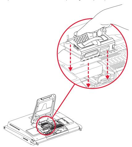
6 Replace the hard disk drive/memory cover by lowering it into place, and sliding it so the slots on the cover fit into the grooves under the computer stand.
