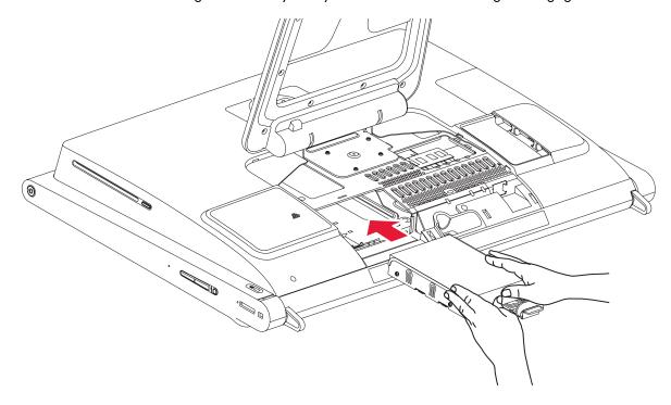
4 Connect the power and data cables to the hard disk drive.
