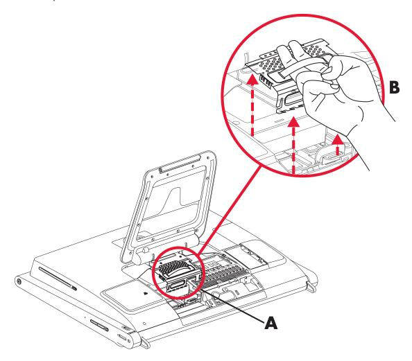
3 While the hard disk drive is still in the computer, disconnect the power and data cables on the hard disk drive, by pressing down the latches and then removing them from the drive.
