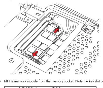
Lift the memory module from the memory socket. Note the key slot on the connector edge.
