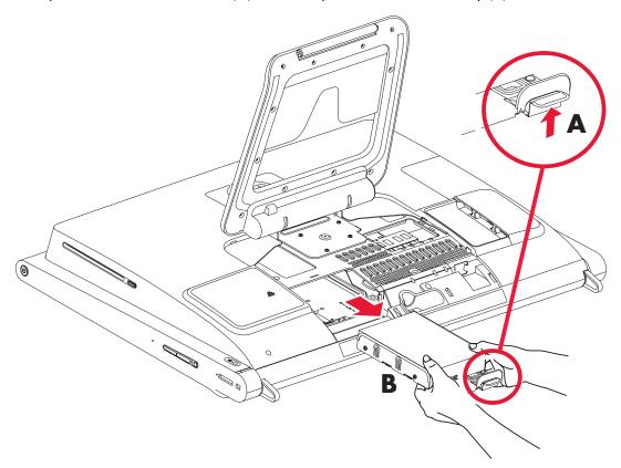
5 With a Phillips screwdriver (magnetic-tipped recommended), remove the four screws that secure the hard disk drive to the cage, and then slide the hard disk drive out of the cage.
