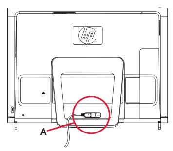
4 Remove the connector cover by inserting your finger under the gap on the bottom-left side of the cover (A), and then pulling gently.
