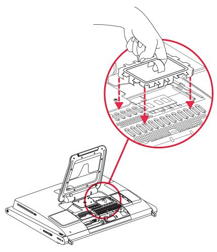
5 Replace the hard disk drive/memory cover by lowering it into place, and sliding it so the slots on the cover fit into the grooves under the computer stand.
