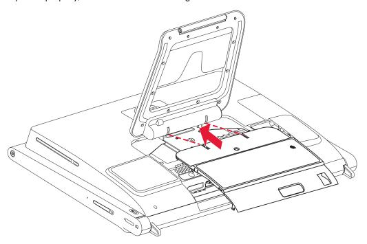
**7** Replace the screw that secures the hard disk drive cage to the chassis.
