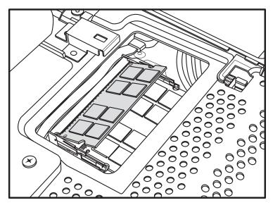
**NOTE:** The sockets are keyed. If the module slot does not match the socket, turn the memory module over.
