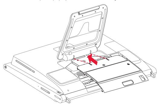
6 Replace the screw that secures the hard disk drive cage to the chassis.
