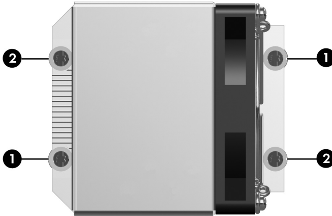
Figure 10 Tightening the heatsink screws
