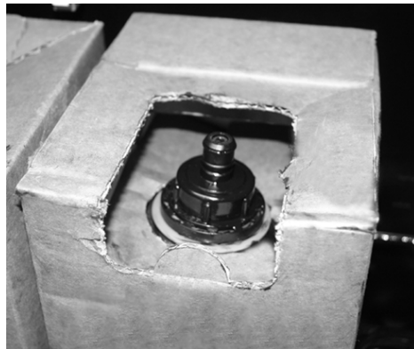
Fig. 3-1. Ink box with supply connector
