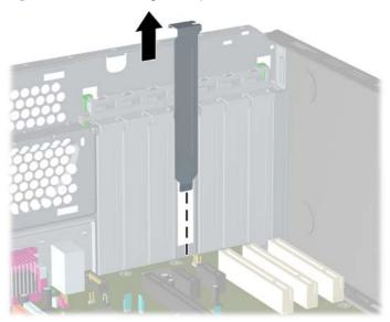
**b.** If you are removing a standard PCI card, hold the card at each end and carefully rock it back and forth until the connectors pull free from the socket. Lift the card straight up to remove it. Be sure not to scrape the card against other components.
