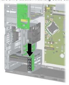
Figure 2-24 Extra Optical Drive M3 Guide Screws Location
