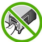
**Cause:** The protective plastic tape was only partially removed from the print cartridge.
