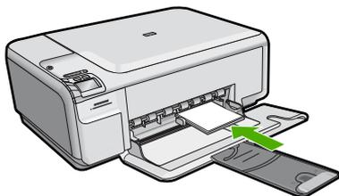
3. Slide the paper-width guide inward until it stops at the edge of the paper. Do not overload the input tray; make sure the stack of paper fits within the input tray and is no higher than the top of the paper-width guide.
