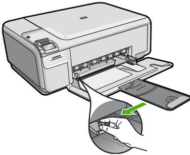
3. Insert the stack of cards into the far-right side of the input tray with the short edge forward and the print side down. Slide the stack of cards forward until it stops.
