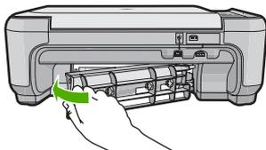
**Cause:** The rear door was not securely installed.
