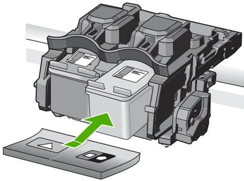
8. Remove the tri-color print cartridge from the slot on the left.
