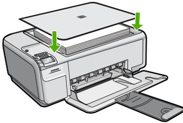
4. When you finish copying or scanning, replace the lid by inserting the tabs on the lid back into the appropriate slots of the product.
