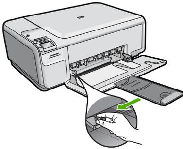
3. Insert one or more envelopes into the far-right side of the input tray, with the envelope flaps on the left and facing up. Slide the stack of envelopes forward until it stops.
