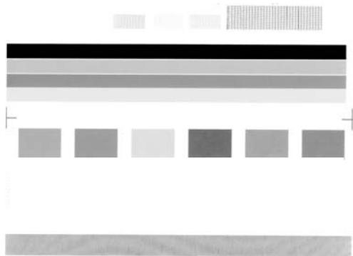
3. Make sure the test patterns show a complete grid and the thick color lines are complete.
