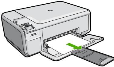
2. Slide the paper-width guide to its outermost position.
