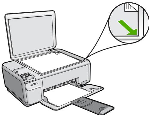
**Cause:** The original was placed incorrectly on the glass.
