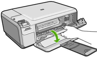
4. Wait until the print carriage is idle and silent. Lightly press down on a print cartridge to release it, and then pull the print cartridge toward you out of its slot.
