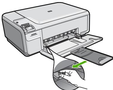
2. Insert the stack of photo paper into the far-right side of the input tray with the short edge forward and the print side down. Slide the stack of photo paper forward until it stops.
