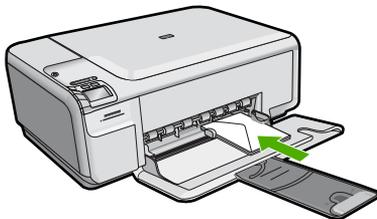
4. Slide the paper-width guide inward against the stack of envelopes until it stops. Do not overload the input tray; make sure the stack of envelopes fits within the input tray and is not higher than the top of the paper-width guide.
