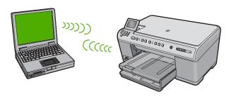
There are two methods you may use to connect the HP All-in-One to your computer using an ad hoc wireless network connection. Once connected, you can install the HP All-in-One software.
