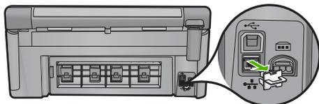
2. Connect the Ethernet cable to the Ethernet port on the back of the product.
