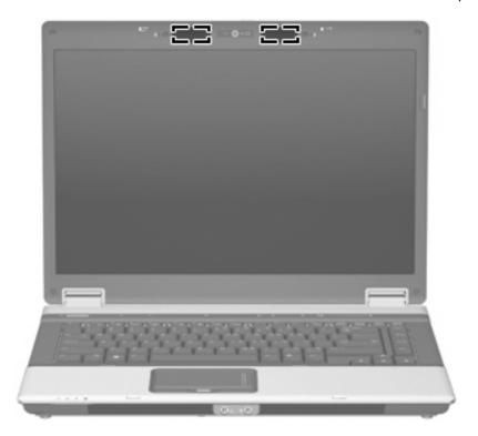
NOTE: For optimal transmission, keep the areas immediately around the antennae free from obstructions.
