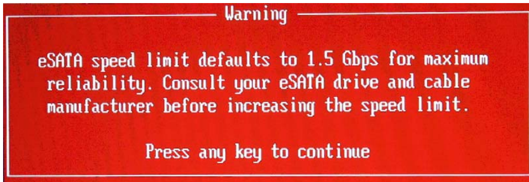
Figure 3 Maximum eSATA speed warning
