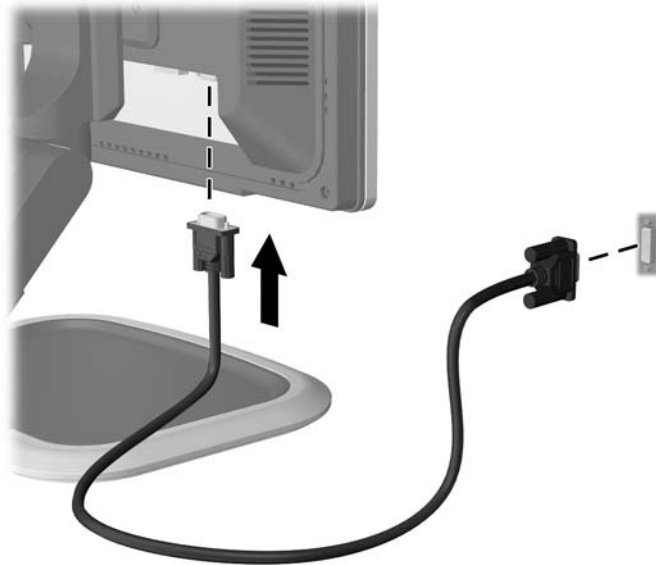
Figure 3-8 Connecting the Signal Cable
