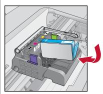
**c.** Turn the ink cartridge over, slide it into the appropriate slot, and then press down until it clicks into place.
