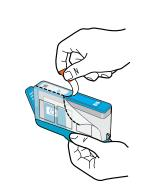
**a.** Remove the plastic wrap by pulling the orange tab.
