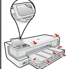
**a.** Remove all tape from the device. Remove the protective film from the display.
