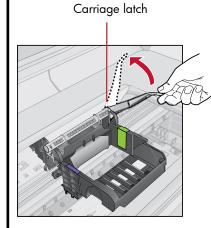
**b.** Firmly lift the gray latch handle, as shown.
