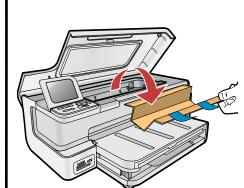
**b.**Open the ink cartridge access door and remove all packing materials from inside.
