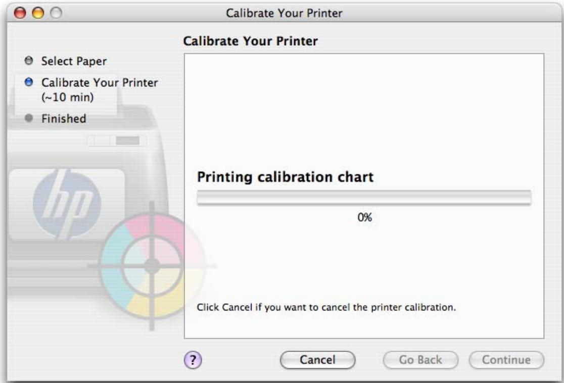
The printer will print and measure this linearization target and calculate the necessary correction factors to apply for consistent color printing on the paper type. It also calculates the maximum amount of each ink that can be applied to the paper.
