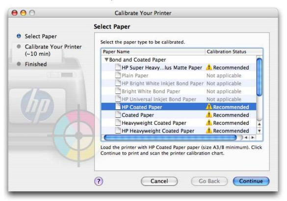
5. A calibration test chart is printed, which contains patches of each ink used in your printer.
