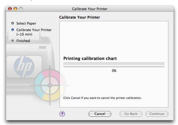
The printer will print and measure this linearization target and calculate the necessary correction factors to apply for consistent color printing on the paper type. It also calculates the maximum amount of each ink that can be applied to the paper.
