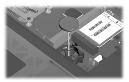
Reverse this procedure to install the RTC battery. Be sure the RTC battery is installed with the "+" sign facing up.
