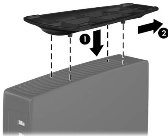
Figure 1-7 Installing the stand
