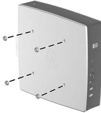
Figure 1-6 Installing the rubber feet
