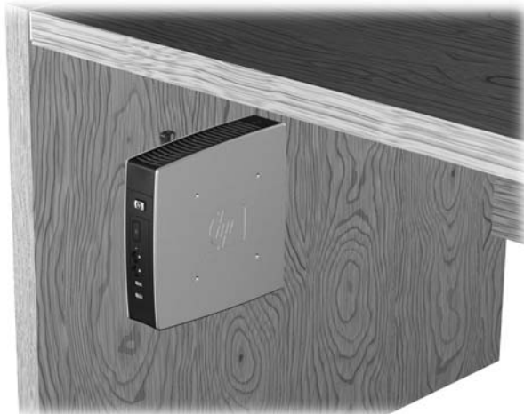
Figure 3-8 Thin client mounted under desk
