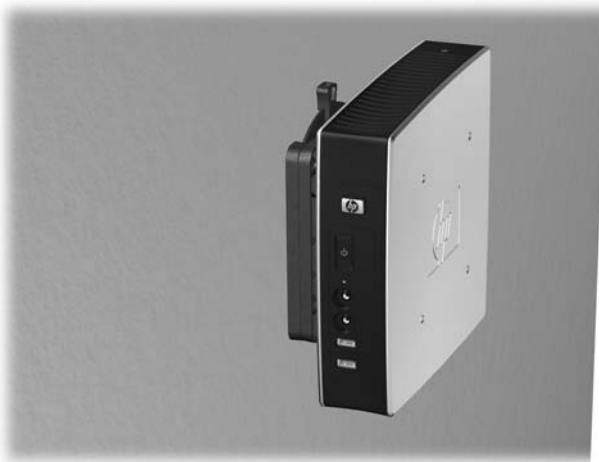
Figure 3-7 Thin client mounted on wall
