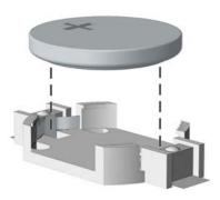
**b.** Slide the replacement battery into position, positive side up. The battery holder automatically secures the battery in the proper position.
