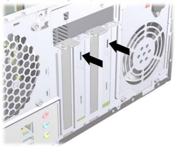
**b.** If you are removing a PCI Express x1 card, hold the card at each end and carefully rock it back and forth until the connectors pull free from the socket. Be sure not to scrape the card against the other components.
