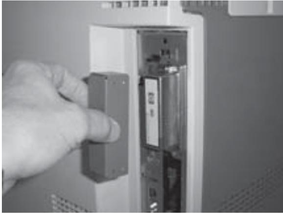
2. Install the optional Kensington-type lock that you purchased for this purpose. (The lock is **not** provided with the EIO lock adapter.)
