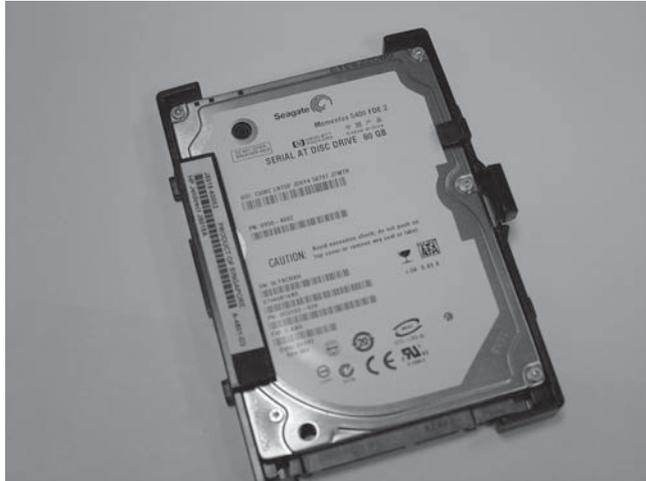
This HP Secure Hard Disk (J8018A) includes pre-mounted disk rails that are typically required for installation in the formatter door.
