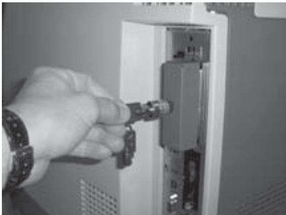
3. Turn to the locked position and remove the key.
