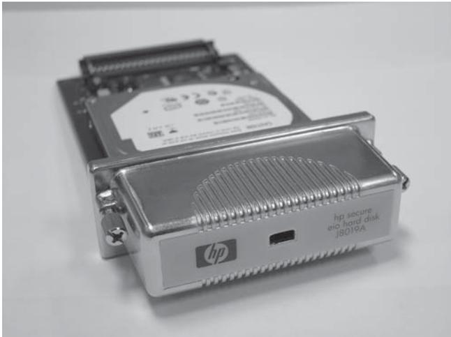
For added physical security, this HP Secure Hard Disk (J8019A) includes an EIO lock adapter (callout 1). The adapter can be outfitted with a Kensington-type lock (with or without a cable). Contact the Kensington Computer Products Group for information about a compatible lock.
