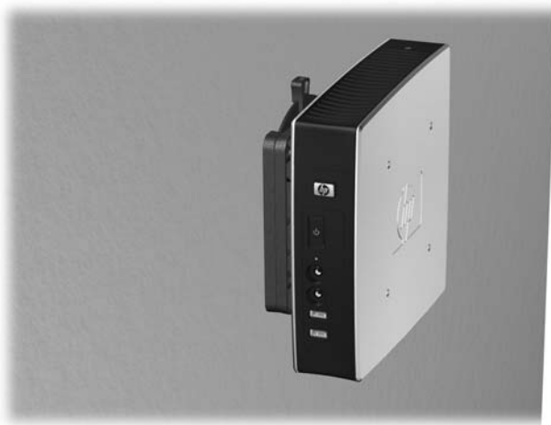
Figure C-7 Thin client mounted on wall
