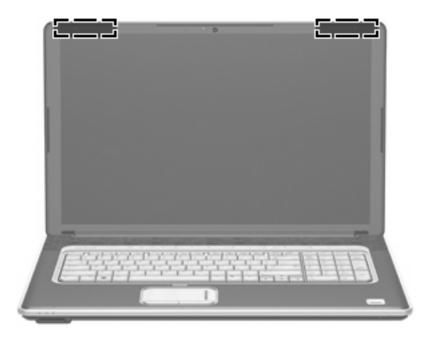
NOTE: The antennae are not visible from the outside of the computer. For optimal transmission, keep the areas immediately around the antennae free from obstructions.
