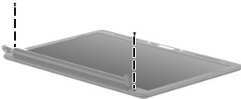
**Where used:** Two screws that secure the bezel to the display assembly
