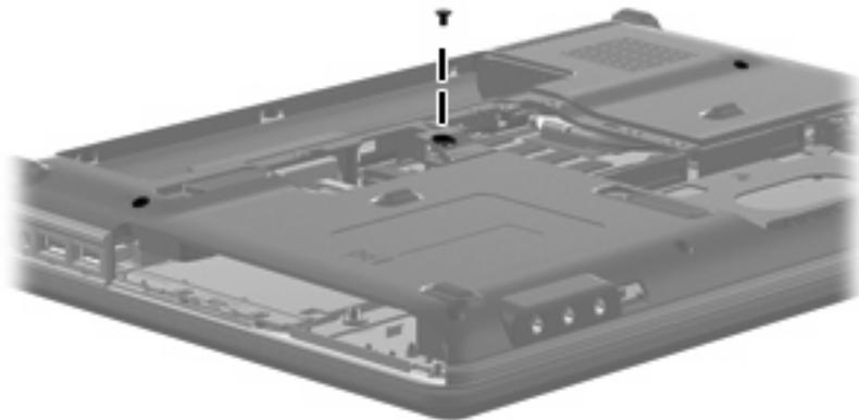
**Where used:** One screw that secures the keyboard to the computer
