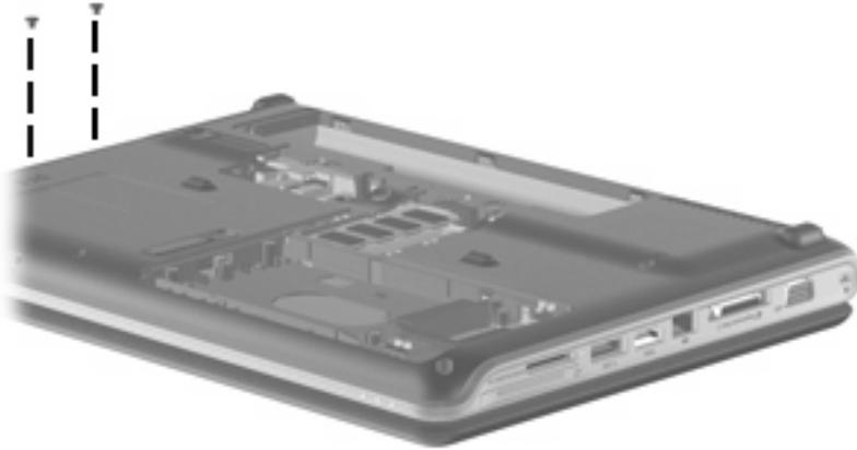
**Where used:** Two screws that secure the keyboard cover to the computer
