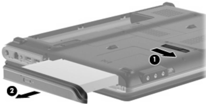
4. If it is necessary to replace the optical drive bracket, position the optical drive with the optical drive bracket toward you.
