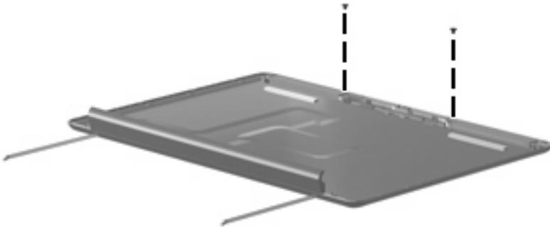
**Where used:** Two screws that secure the wireless antenna transceivers to the display enclosure
