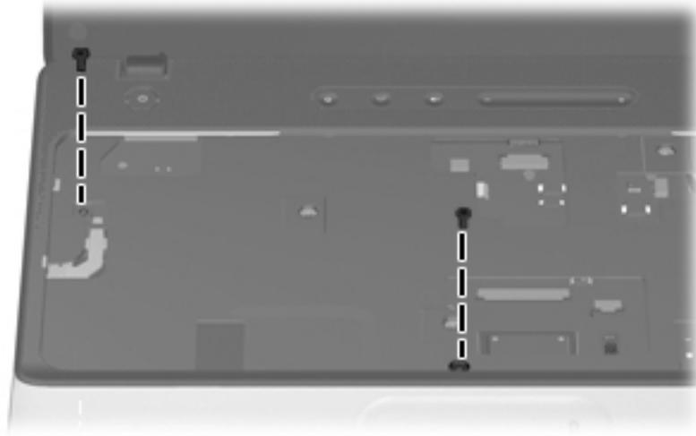
**Where used:** 2 screws that secure the top cover to the base enclosure (top)
