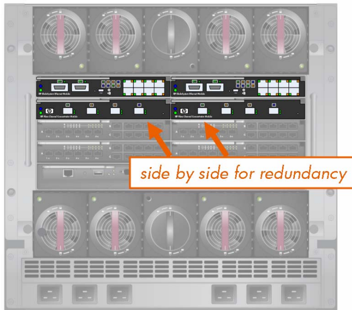
Figure 3. Rear of HP BladeSystem c7000 Enclosure showing redundant Virtual Connect modules
