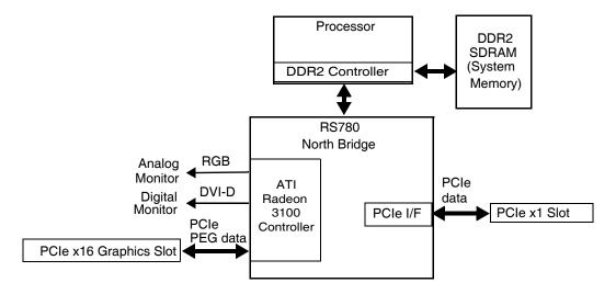
Figure 6-1. Integrated Graphics Processor, Block diagram
