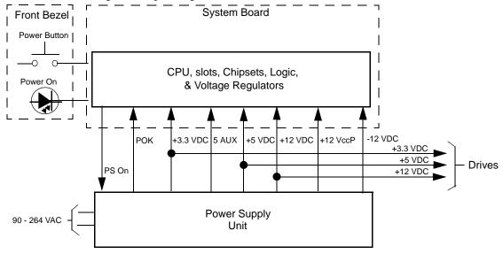
Figure 7-1. Power Generation Block Diagram
