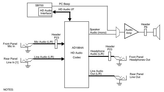
L/R = Separate left and right channels (stereo). L+R = Combined left and right channels (mono). [1] Can be re-configured as Microphone In
