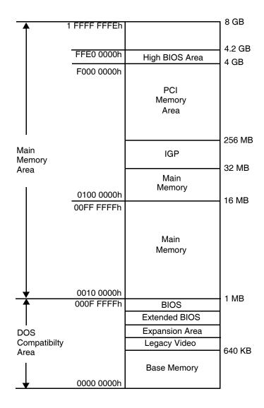
Figure 3-2. System Memory Map (for maximum of 8 gigabytes)
