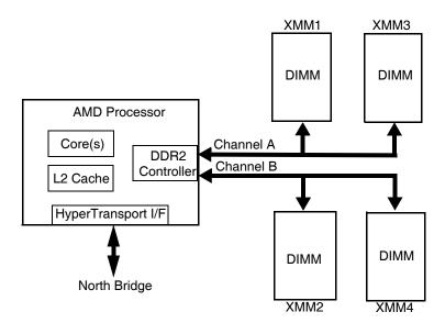
Figure 3-1. Processor/Memory Subsystem Architecture
