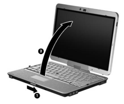
2. Rotate the computer display clockwise until it snaps into place facing away from the keyboard.
