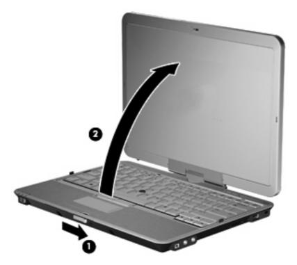
3. Rotate the computer display counterclockwise until it snaps into place facing the keyboard.
