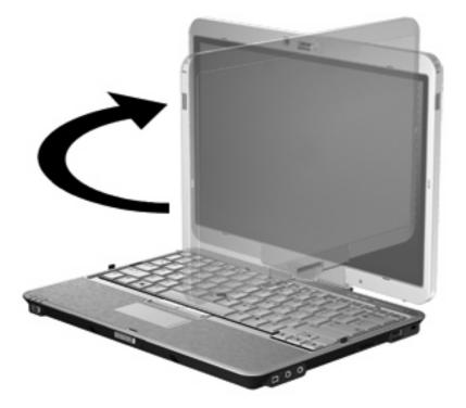
3. Tilt the computer display downward onto the keyboard until it snaps into place.
