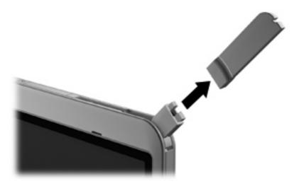
To connect the external WWAN antenna:
