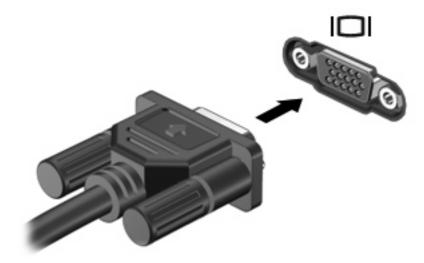
NOTE: If a properly connected external display device does not display an image, press fn+f4 to transfer the image to the device. Repeatedly pressing fn+f4 alternates the screen image between the computer display and the device.
