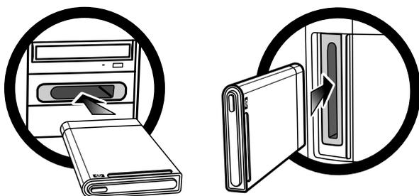
To insert the HP Pocket Media Drive into a specially designed HP computer:
