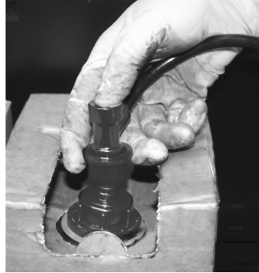
Fig. 3-2. Connecting the ink tube to the ink box
