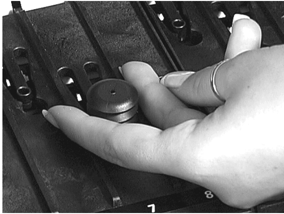
Fig. 5-5. Inserting the priming bulb
