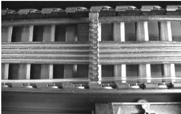
Tube guides inside the tube chain (shown empty with cable)
