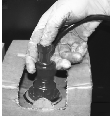
Fig. 3-3. Connecting the ink tube to the ink box
