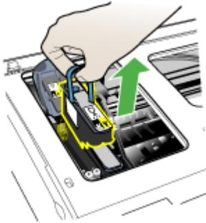
5. Before installing a printhead, shake the printhead up and down at least six times while the printhead is still in its packaging.
