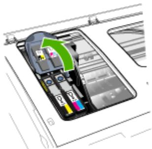
4. Lift the handle of the printhead (which corresponds to the control-panel message) and use it to pull the printhead out of its slot.
