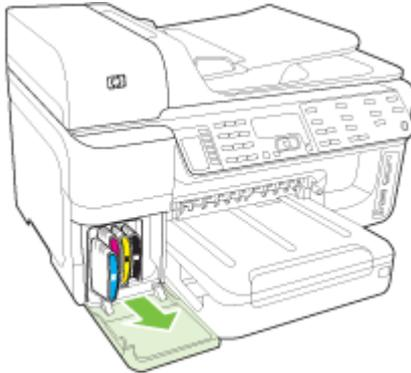
4. Place the ink cartridges in an airtight plastic container so they will not dry out, and put them aside. Do not send them with the device unless the HP customer support call agent instructs you to.
