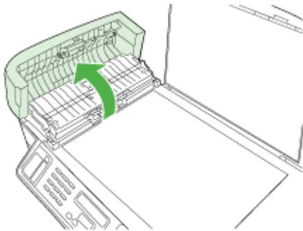
4. Lift the automatic document feeder mechanism, using the two hand grip areas in the front and rear of the device.
