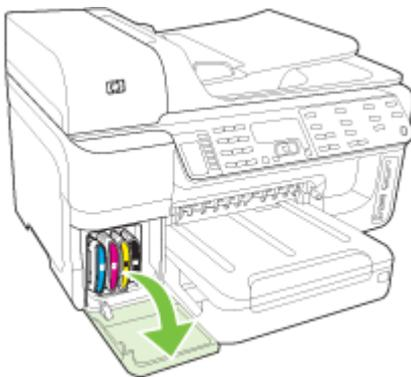
3. Remove the ink cartridges from their slots by grasping each between your thumb and forefinger and pulling it firmly toward you.
