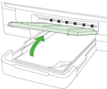
2. Insert the media print-side down in the center of the tray. Make sure the stack of media aligns with the line on the width guide, and is not higher than the paper stack line on the guide.
