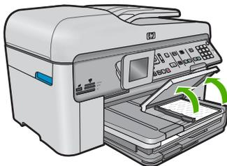
2. Slide the paper-width guide to its outermost position.
