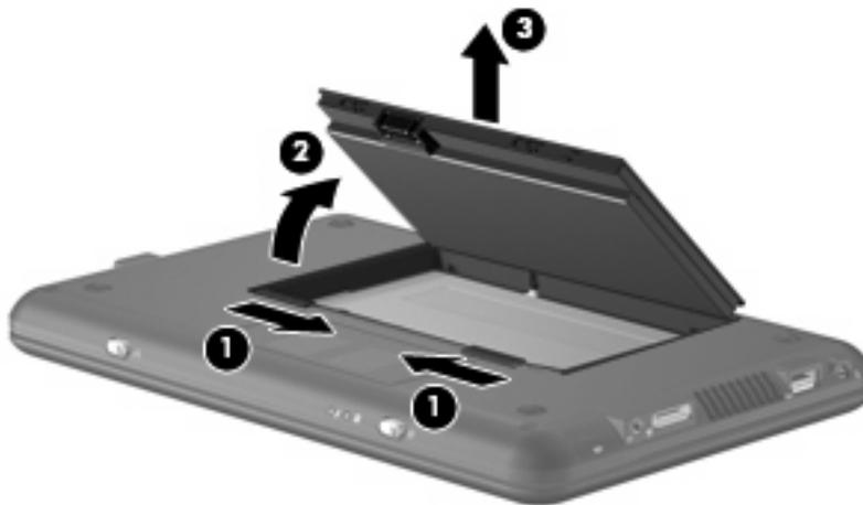
To install the battery, insert the rear edge of the battery into the battery bay and pivot the battery downward until it is seated. The battery release latch automatically locks the battery into place.
