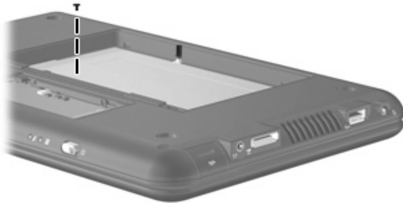
**Where used:** One screw that secures the keyboard to the device
