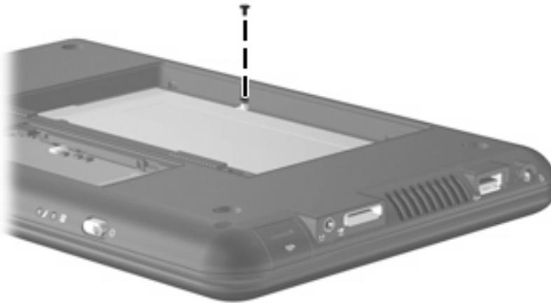
**Where used:** One screw that secures the keyboard to the device
